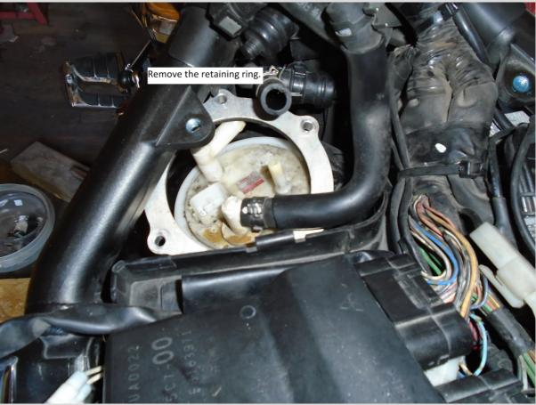
Grab the pump housing and start pulling it up and out of the sub-tank. You will need to tilt the sub-tank to the right, while wiggling and rotating the housing to get it to clear the frame. Go slow and pay attention to the housing's position as you pull it out. This will be very helpful when it's time to reinstall it.
