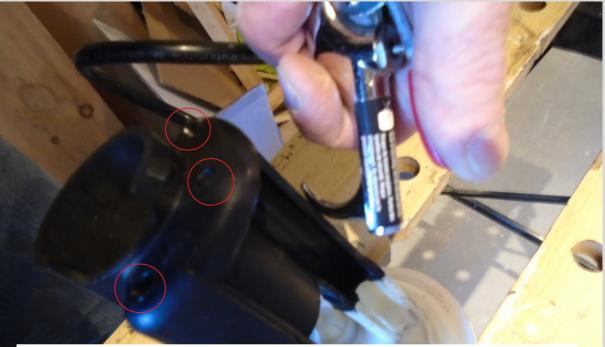
When you're done with the cutting and drilling,it's time to clean up your work. De-burr the edges,remove any bits of loose plastic,etc. Thoroughly wash/dry the housing. Remember,this is going inside the fuel sub-tank. Any loose particles will end up in the fuel pre-filter at the pump inlet. You don't want it to clog. I used dish soap/water and an old toothbrush to wash my housing,and compressed air to dry it.
