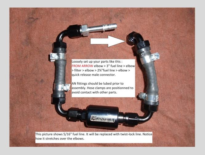
Remember: Do not use the SAE 30R10 submersible fuel line here. Use only regular FI rated fuel line.
