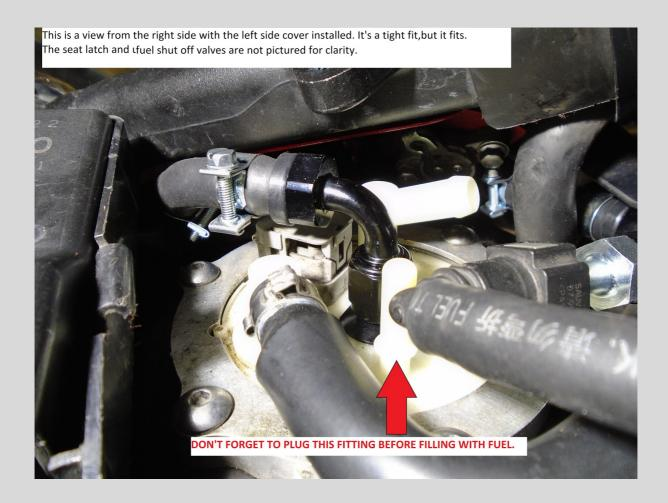
Reinstall the fuel tank, connect the lines and open the shut off valves. Before adding any fuel to the system, plug the old fuel pressure fitting on the housing. I used a piece of FI fuel line with a bolt inside and 2 clamps. I don't recommend using carburetor vacuum port plugs because they were designed for vacuum, not fuel. They will deteriorate from fuel contamination over time.
