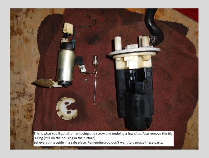
Now we'll start cutting into the housing. At this point, unless you've been letting it air out a few weeks, the housing still has fuel inside. Again avoid sparks and open flame.
