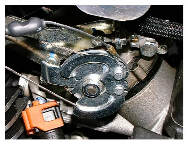
16. Lay the servo cable in the track on the bellcrank.
