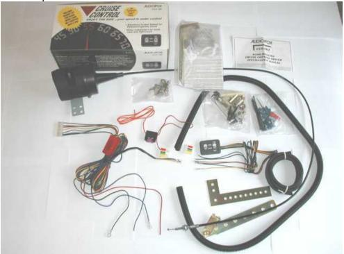
3. You can remove the gray and black wire pair from the 10-pin connector since it will not be needed.
