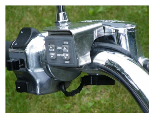
25. After you are satisfied with your bracket, you might need to lengthen your wires from the control unit. Temporarily mount the control switch to the bracket but don't peel the backing off the mounting tape. Use a rubber band to hold the control in place.
